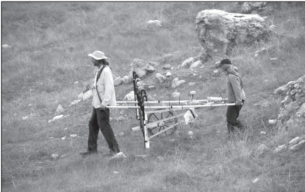
2. The challenging surface conditions of Jarash's southwest district are characterised by field obstacles such as rocks, piles of stones and steep slopes. Photo shows seven Fluxgate Förster Gradiometer FEREX CON650 sensors mounted on a portable array. © LAJP.
